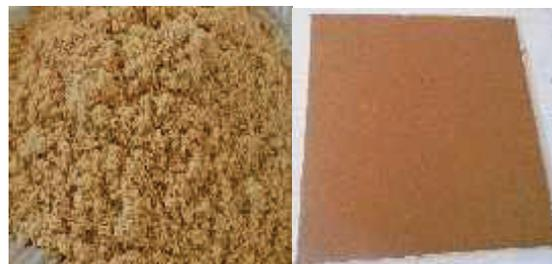
Figure 1. The manufactured wood plastic composites
