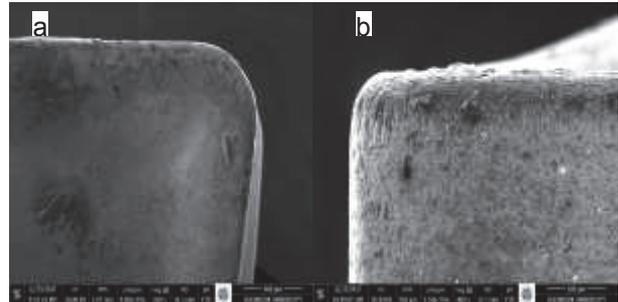
Fig 3.5. 10 nm  $\text{Al}_2\text{O}_3$  coated Cementite Carbide Cutting tool with a cutting speed of 120 m / min, a) top view; b) the cutting side surface
