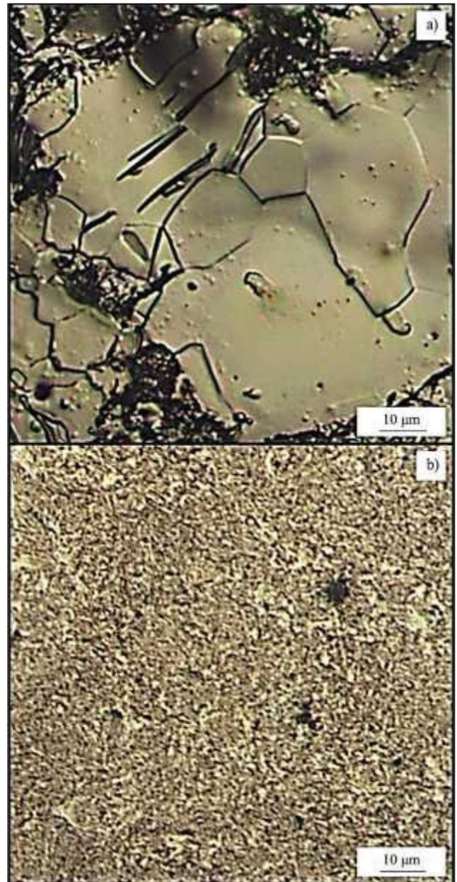
Fig. 4 Microstructures of matrix of sintered samples a) as-received b) milled
