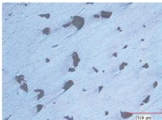
Fig. 2 Microstructure of the composite sample containing 5 vol. %  $\text{Al}_2\text{O}_3$ , after sintering at 600 °C.
