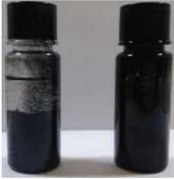
Fig. 5 Stability of MWCNT dispersions a) t:1 hour b)2 hour (a:MWCNT, surfactant,ethanol b:MWCNT,surfactant,resin)
