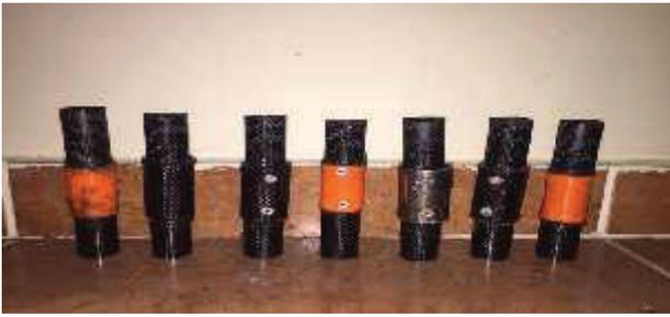
Fig. 1. Carbon epoxy composite tubes combined to different types of joint materials by multiple rivets, epoxy glue and both of them.
