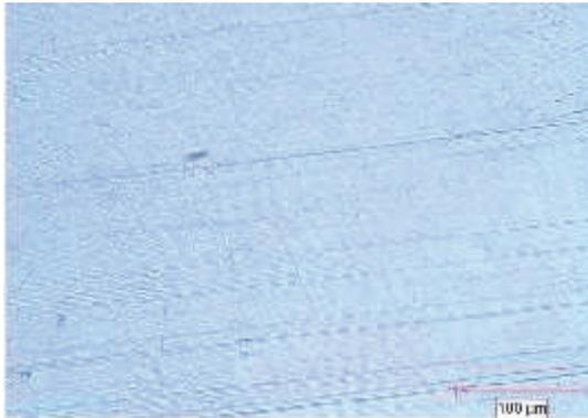
Fig. 1 Microstructure of the Al-4%Cu matrix alloy, after sintering at 600 °C.
