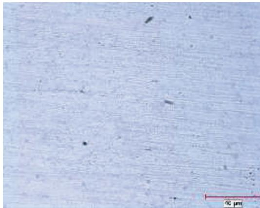
Fig. 1 Microstructure of the Al4Cu alloy, sintered at 610 °C
