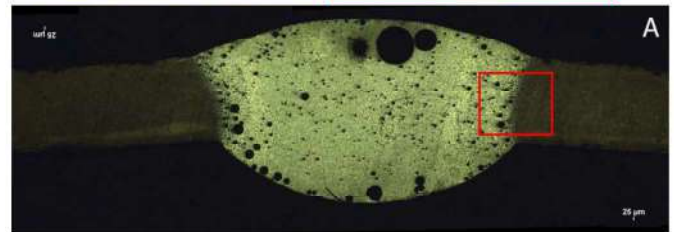
Fig. 5 Sample A macro weld metal and HAZ optic images.
