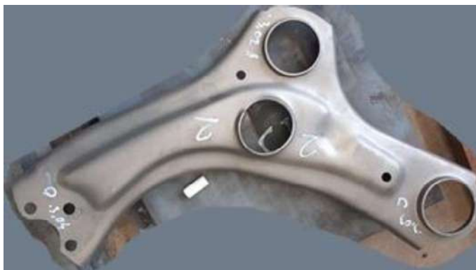
Figure 2. Comparison of the fatigue behavior on the press hardened control arm for the different materials.
