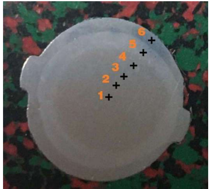
Figure 3.1. Points where hardness test is taken from B420C ribbed reinforced concrete steel.
