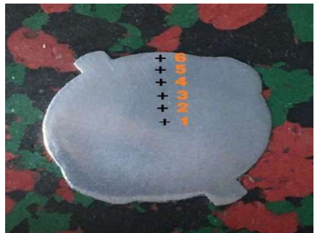
Figure 3.2. Points where the hardness test is taken from S420 ribbed reinforced concrete steel.
