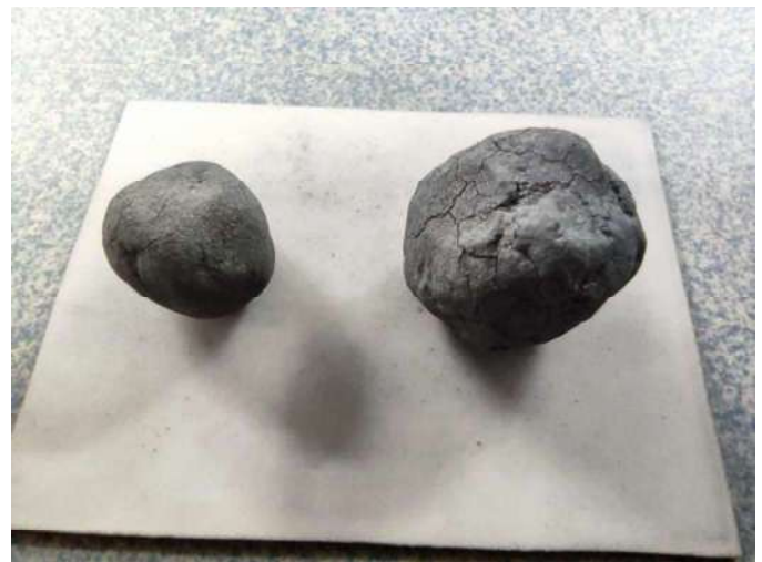
Fig. 13 Pellets reduced in hydrogen at 1000°C.
