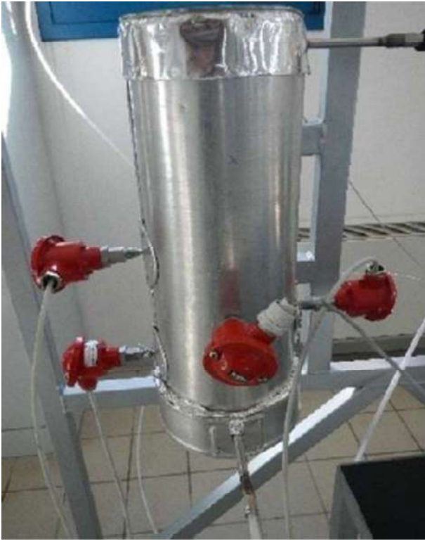
Fig. 3 Customized shaft furnace.
