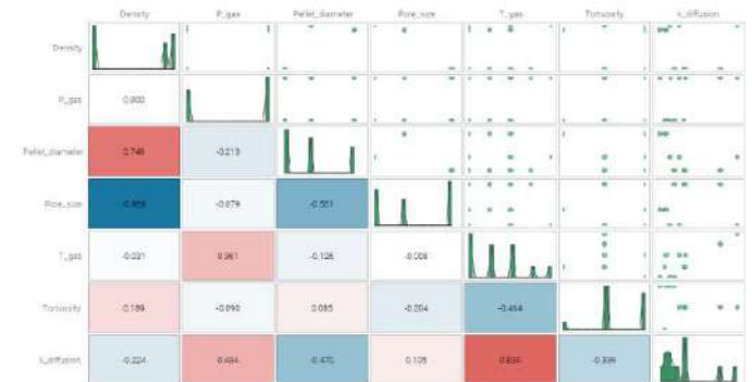
Fig. 21 Scatter matrix relative to the dependence of the kinetic parameter (Eq. 2) on the different input parameters.
