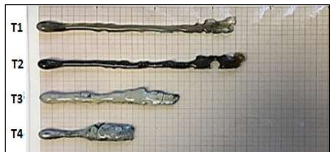
Fig. 6 The ribbons of T-series mould powder from the inclined plane test.
