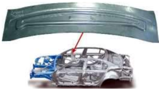
Fig. 2 Location of the roof stiffener sheet on the vehicle
