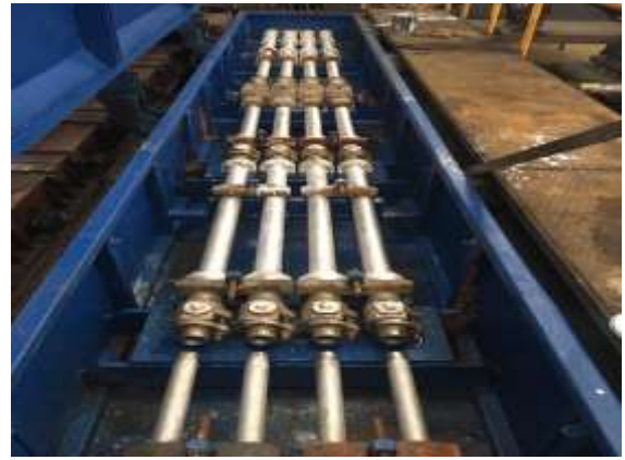
Fig. 3. Tempcore Cooling System [5]
