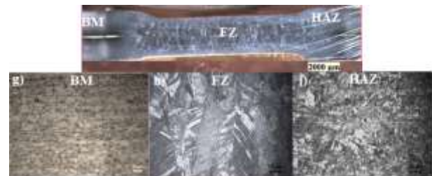
Figure 4. The weld zone profile and its microstructures of DP600 weldment joined with 5.5 Bar electrode force with 4kA welding current. a) Base metal (BM), b) Heat Affect Zone (HAZ), c) Fusion zone (FZ).
