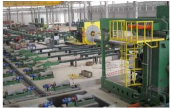
Fig. 1 Material handling system (pipe transfer systems)
