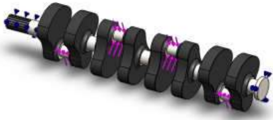
Fig. (4) Boundary Conditions of the Designed Model
