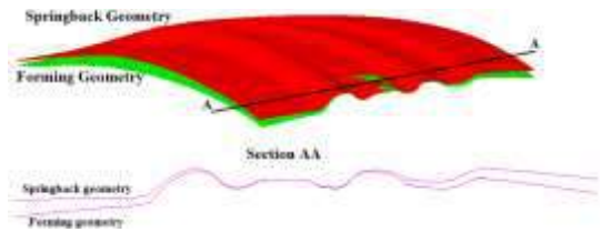
Fig. 5 Forming and springback geometries obtained by finite element analyses
