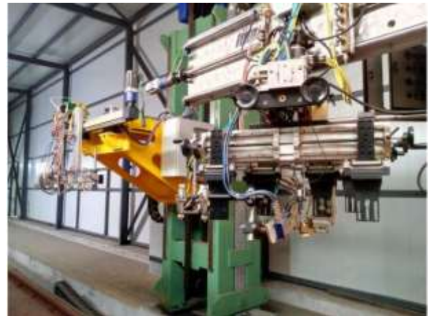
Fig. 2 Ultrasonic testing system
