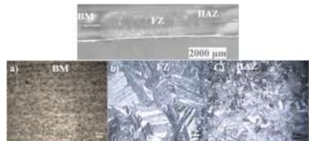
Figure 5. The microstructure of weldment joined with 3.5 Bar electrode force with 8kA welding current a) DP600 base metal (BM), b) DP600 Heat Affect Zone (HAZ), c) DP600 Fusion Zone (FZ)
