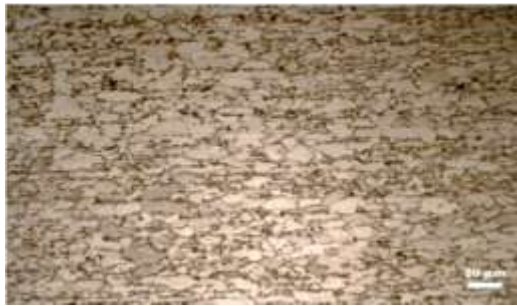
Figure 1. Microstructure view of DP600 steel.
