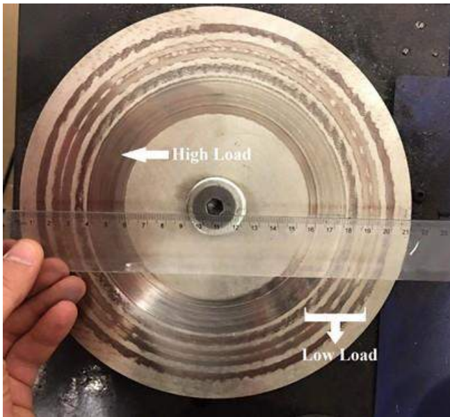
Fig.6 Macro view of low and high load wear on the counter disk.
