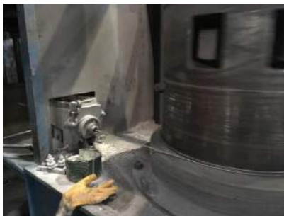
Fig. 3: The wire is passing on the first drawing head
