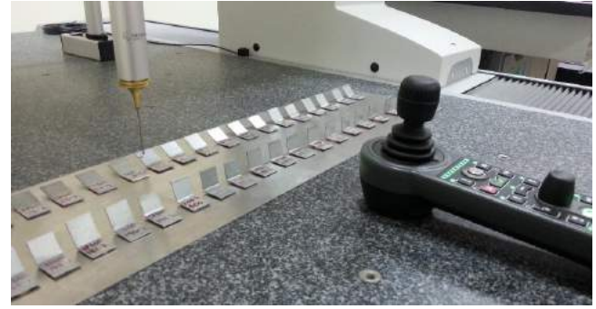
Fig. 3 The springback measurement by CMM
