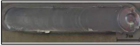
Fig. 4 Macrograph of the FSPed zone of TRIP Steel
