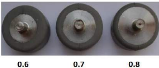
Fig. 5 Samples which have outer diameter of 20 mm and D_i/D_m ratio of 0.6, 0.7 and 0.8
