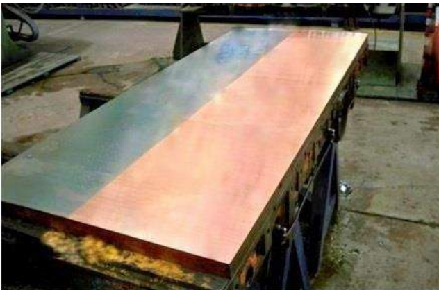
Fig. 2 Nickel-coated mold wall
