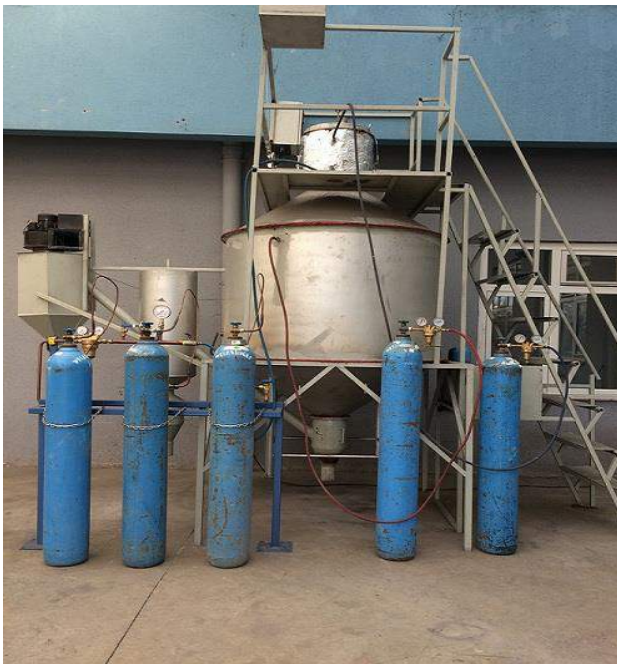
Figure 2. Karabük University Gas Atomization Unit
