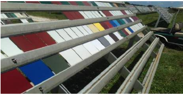
Fig.4 MMK Metalurji samples at natural weathering test area in Florida
