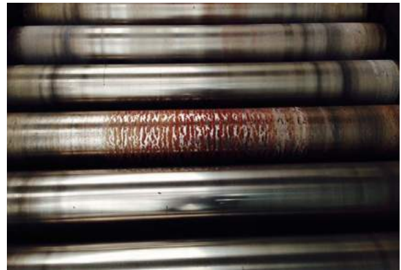
Fig. 3 Appearance of corrosion beginning in ECR.
