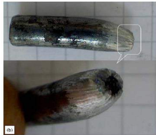
Fig. 7 Damage on the projectile tip after impacting (b) plastic deformation of the tip by bending.
