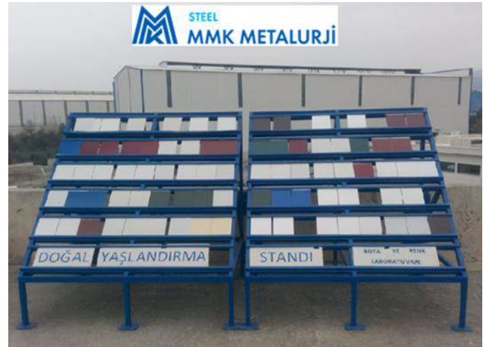
Fig.5 MMK Metalurji samples at natural weathering test area in Dörtyol/Hatay/Turkey
