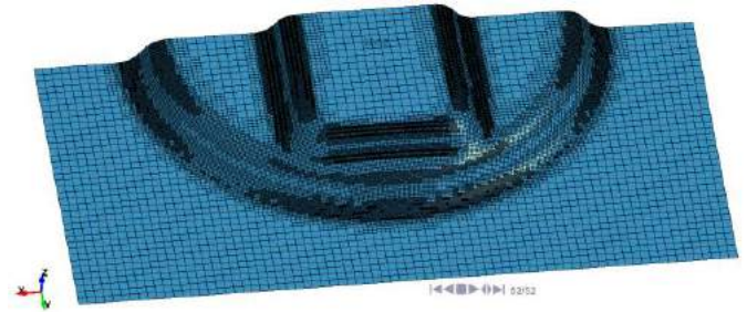
Fig. 4. Mesh structure after remeshing for hydroformed AHSS sheet
