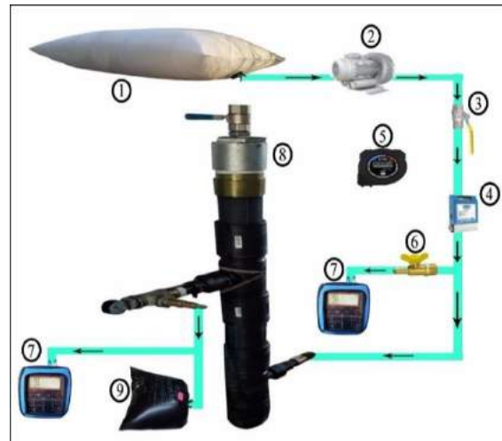
1 Soft tank 4 Gas flow meter 7 Biogas analyzer 2 Blower fan 5 Digital stopwatch 8 Purification tower 3 Flow regulator 6 Sample valve 9 Sample Container
