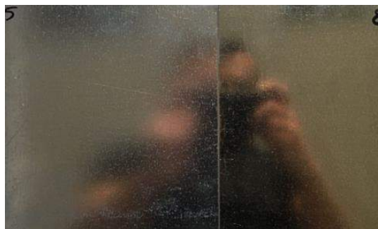
Fig. 3 A photo of a dull and a shiny galvanize samples
