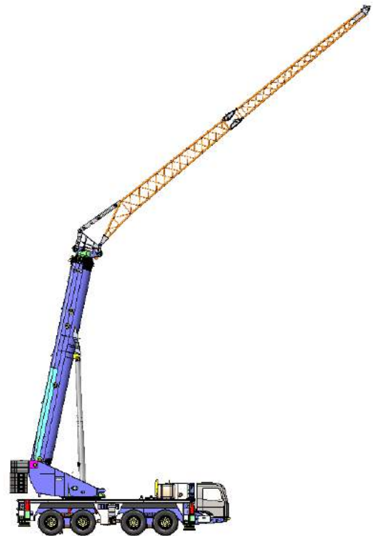
Fig.3 Mobile crane design
