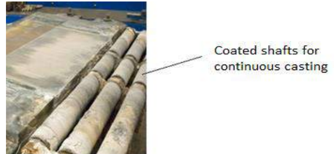
Fig. 32 The coated shaft after use
