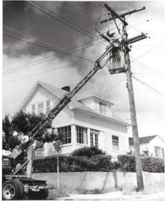
Fig.1 An aerial work platform designed by Eitel in 1944
