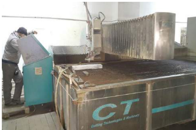
Fig. 1. Waterjet machining system used in this study
