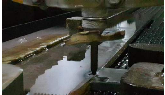
Fig. 2. An image from the machining of A356 aluminium alloy on the waterjet lathe.
