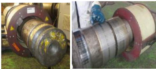
a) Heating of the ring b) Extracting of the ring
