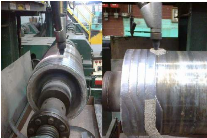
Fig. 31 Shaft coated with submerged arc welding method
