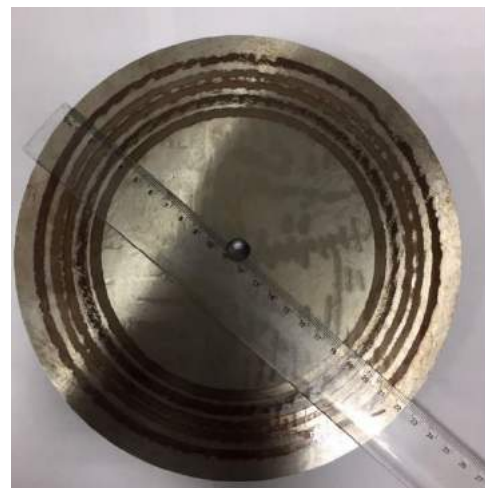
Figure 7. Wear Tracles on of the Counter Disc after Wear Test
