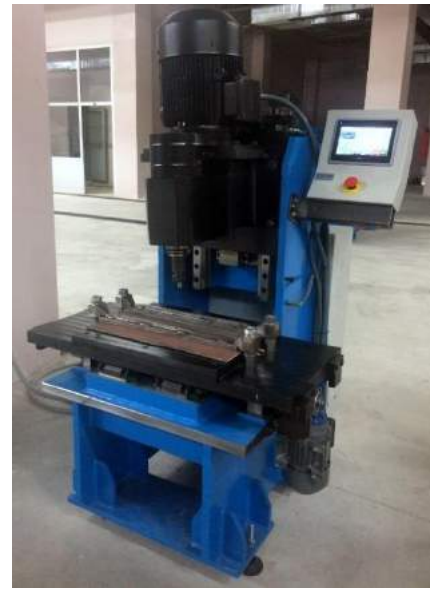
Fig. 2. Photograph of Friction stir processing/welding test rig used in the study.
