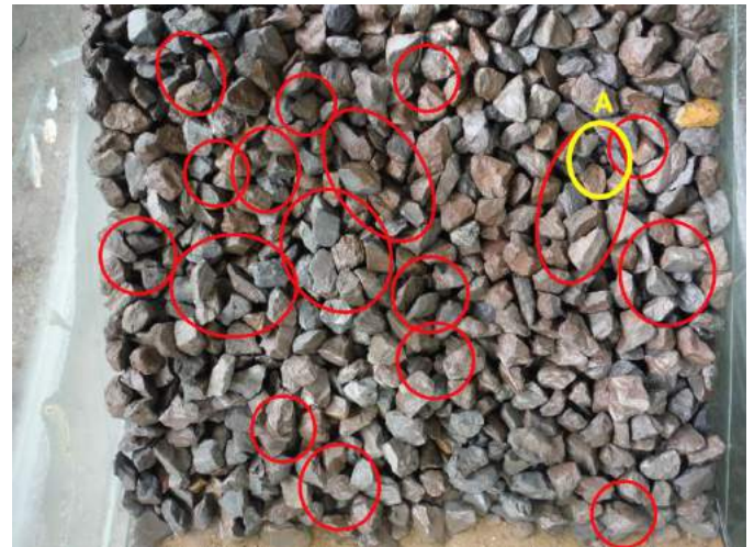
Fig. 17 A sample after-the-test photo that shows the damage on the armour layer due to wave attack.
