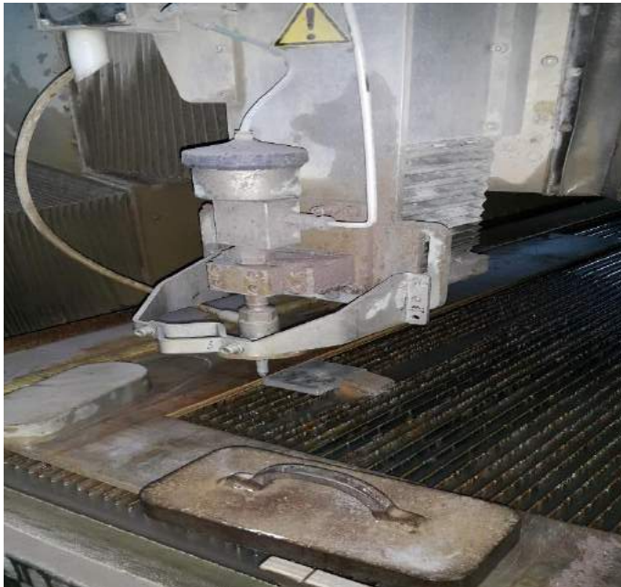
Fig. 1. AISI 316 stainless steel sample being machined.
