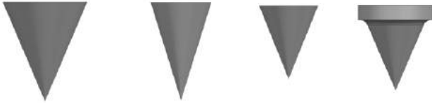
Fig. 8 The pouring basing geometries of Line 7 - 6 - 3 - 2, respectively
